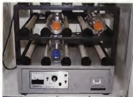
16-9, 10 Roller bottles. Roller bottles are also utilized for growing large quantities of viruses in cell monolayers (Figure 16-9). The cells are seeded into the bottle with medium and the bottles are placed in a roller bottle apparatus (Figure 16-10) located inside an incubator that continuously rotates the bottles. Once the cells are attached in a monolayer around the interior walls of the bottle, the viral inoculum is added and the bottle placed back on the rotating module (New Brunswick Scientific, Edison, N. J.). The cells can be harvested when the desired CPE is observed in the cell monolayer.
